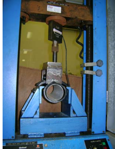
Fig.4 Compression method of testing the saddle/pipe joint sample
