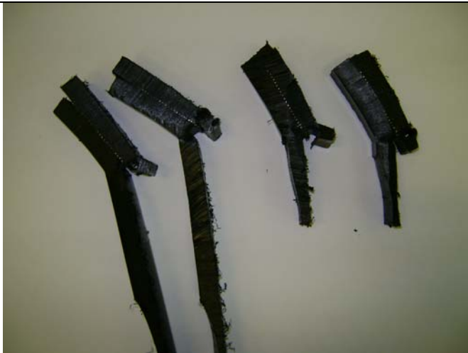
Fig. 5 Fusematic cap/pipe joints failed in ductile mode
