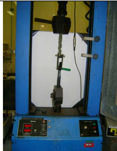
Fig.6 Tensile method of testing the cap/pipe joint samples
